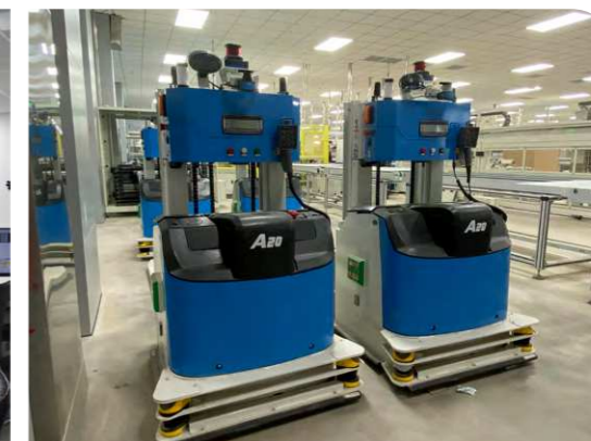
电池、组件基地AGV系统 AGV system for both the cell and module manufacturing bases
